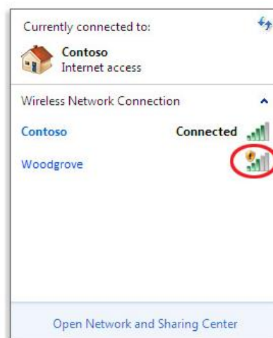
Connect to a Network, showing the shield icon on an unsecured network
