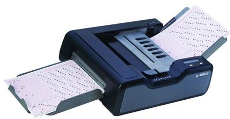
The OMR device can detect ordinary pencil and pen marks made on special pre-printed cards or forms by sensing reflected light. In order to be detected the marks have to be placed in a special position. This device is suitable for handling questionnaires and multiple choice examinations. Information is collected on a pre-printed OMR form by making pre-determined positions with a pencil or pen to indicate each selected response.
