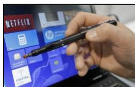
A light pen is a light-sensitive computer input device, basically a stylus, that is used to select text, draw pictures and interact with user interface elements on a computer screen or monitor.
