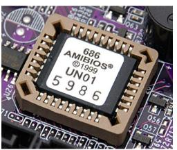
bootstrap loader which allows the computer to start-up (load the Operating System into RAM) when the computer is switched on. Unlike RAM, ROM is non-volatile, data is not lost when the power is switched off. In short, ROM is:
