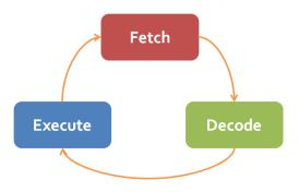
fetching, decoding, and executing an instruction is continually repeated by the CPU whilst the computer is turned on.
